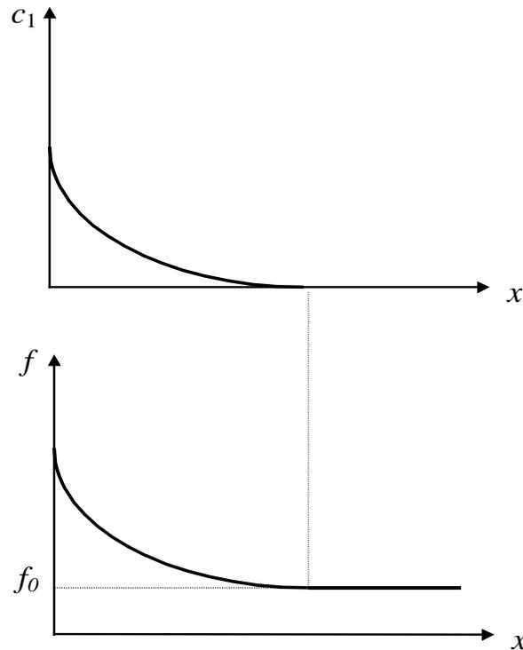
Fig. 5: Schematic presentation of spatial profiles of the oxygen concentration  $c_1(x)$  and hydride distribution function  $f(x)$  in the metal cladding.
