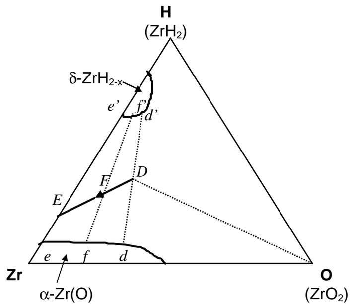
Fig. 3: Schematic ternary Zr-O-H phase diagram with the diffusion path *DE*
