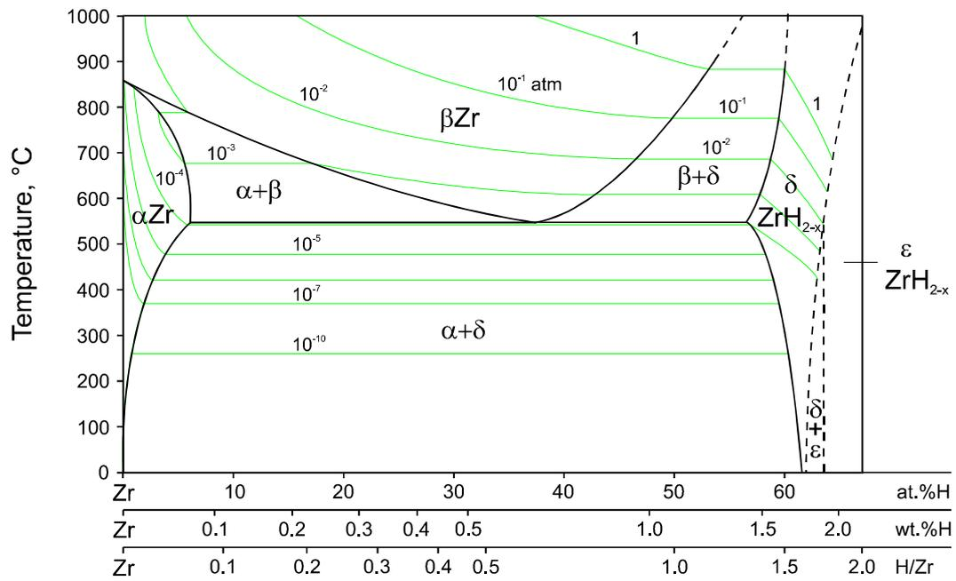
Fig. 4: Binary Zirconium-Hydrogen phase diagram and equilibrium hydrogen pressures (from [15]).
