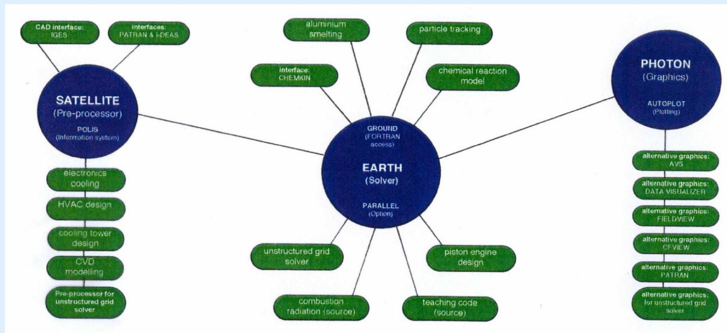
Modular design: central solver, pre-processor (mesh generator), post-processor (graphical display of results) and modules to link in, as needed for the application.
