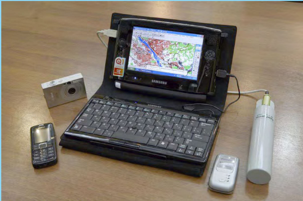
Compact laptop with GPS and gamma-sensor
